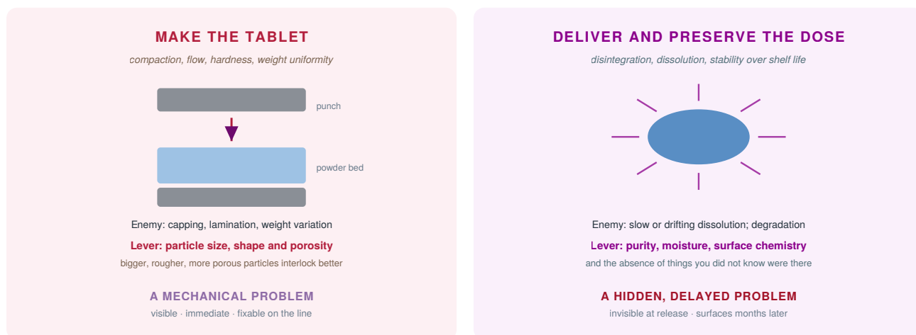
Figure 2.1 — The two problems. The tablet must be strong enough to survive manufacture and shipping, and weak enough to fall apart on schedule inside a patient. They are tuned by different levers, and they fail in completely different ways.
